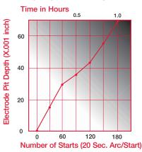
(2) Electrode erosion of .060" is typically end of electrode life.
